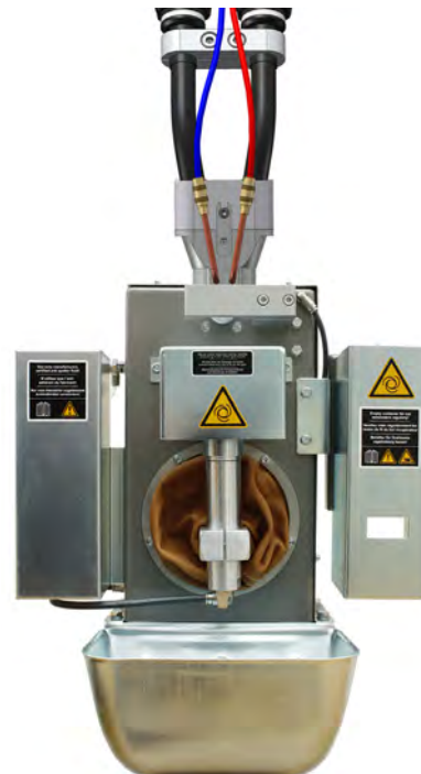
Robot with mounted Dinse Tandem torch head during the cleaning in the Tandem torch cleaning station
