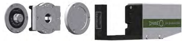
Storage station with fixture mandrel, tool holder and SAS - flange
