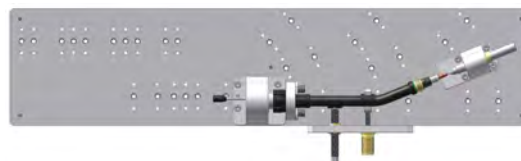
Checking jig PV 200 XL converted to the straightening device with support set DIX PVS 102, aligning bracket JH 100, torch dapter DIX PVP 102 and straightening set PVR 102
