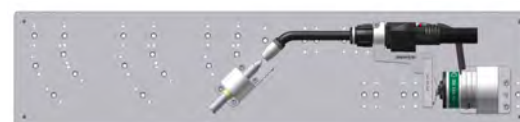
Checking jig PV 250 XL with complete torch system, separable, torch bracket, fixed and shock sensor DIX SAS 100
